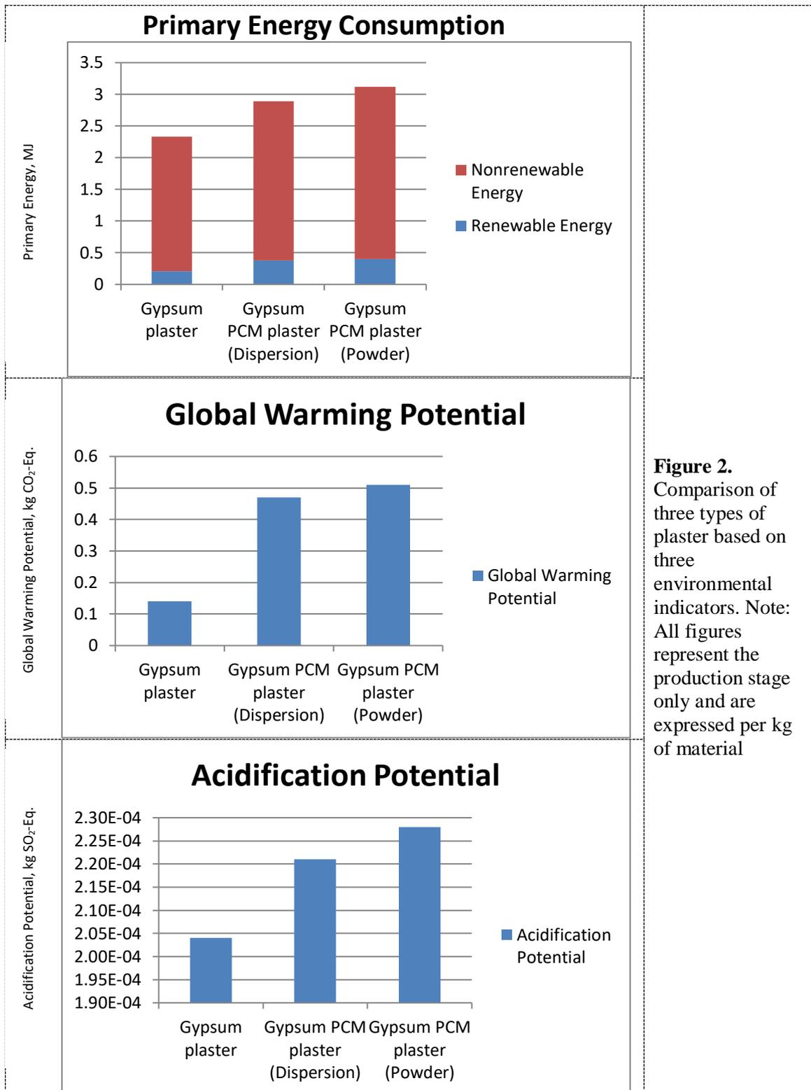
**Figure 2.** Comparison of three types of plaster based on three environmental indicators. Note: All figures represent the production stage only and are expressed per kg of material
