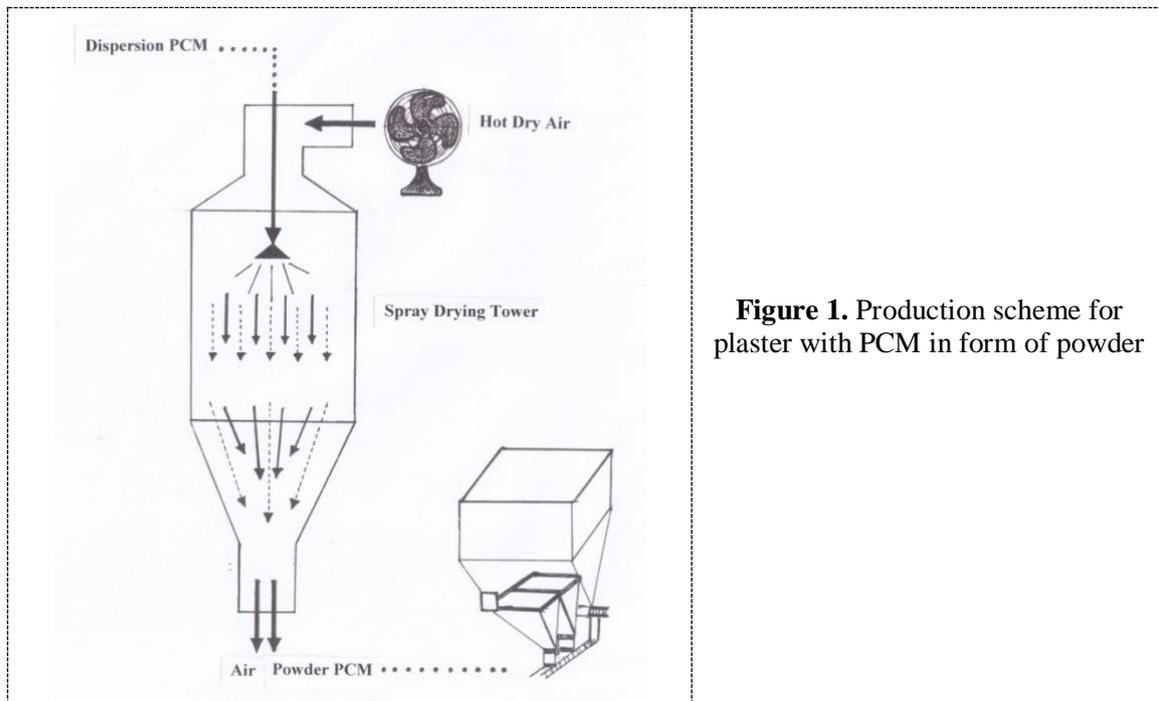
**Figure 1.** Production scheme for plaster with PCM in form of powder
